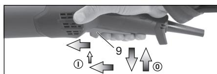
**Switching on:** Switch the machine on as described above. Now slide the trigger switch (9) forwards again and release it in the front
