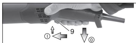
**Switching on:** Slide the trigger switch (9) forwards and then push the trigger switch (9) upwards.
